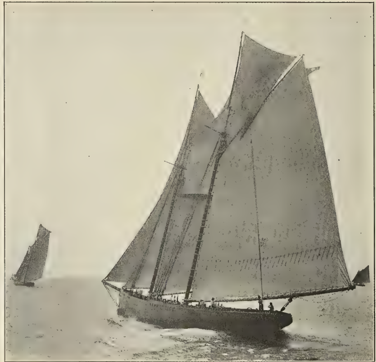
A GOOD SAIL, SHOWING DRAFT IN LUFF. ROSE DOROTHEA. (Photographs by N. L. Stebbins.)
